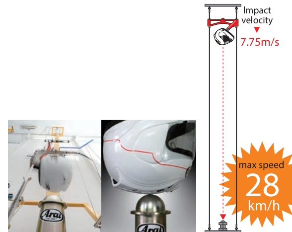
As for the force involved, if you convert the force from the helmet drop test of the strictest helmet standard in the world, it amounts to merely 27.9km/h (or 7.75 m/s).
